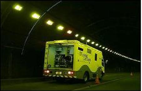
Tunnel inspection using High-Speed Concrete-crack Measurement Vehicle
