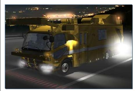
Pavement inspection using High-Speed Road Measurement Vehicle
